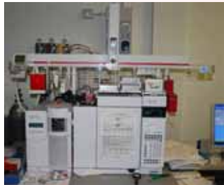
Agilent 5975C MSD spectrometer with Gerstel MPS2 XL equipped with SPME option
