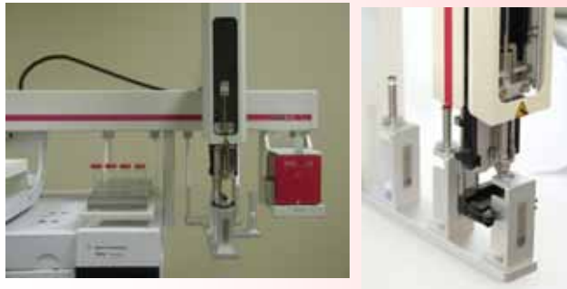
Agilent 5975C MSD spectrometer with Gerstel MPS2 XL equipped with SPME automatic fiber exchange option
